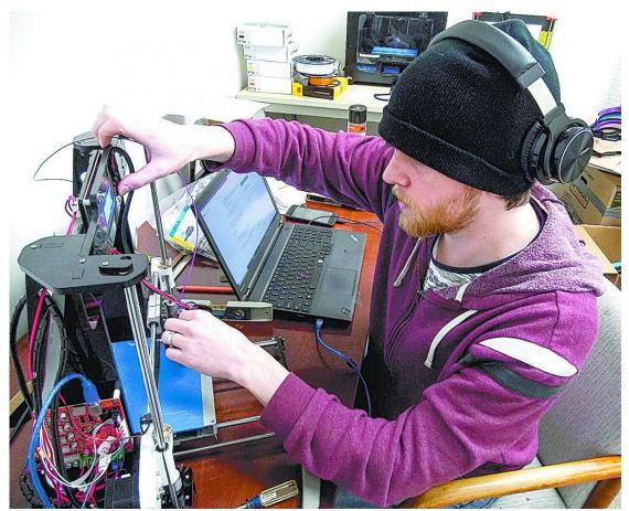
Photos courtesy of Lipofskyphoto.com Dan Bower works at a 3D printer to make components of a plastic mask.
